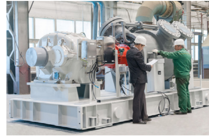
Gas compressor package on the basis of the 25MW 5GC2-287/15-57 GTU compressor
